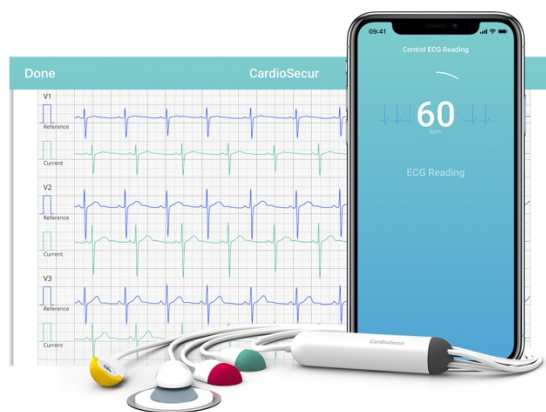
CardioSecur records a clinical-grade ECG with up to 22-leads and only 4 electrodes. ©CardioSecur
